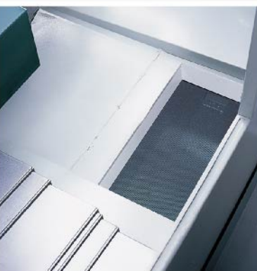
Integrated sheet metal fabrication, with large chip disposal openings, contributes to convenient chip cleaning.
